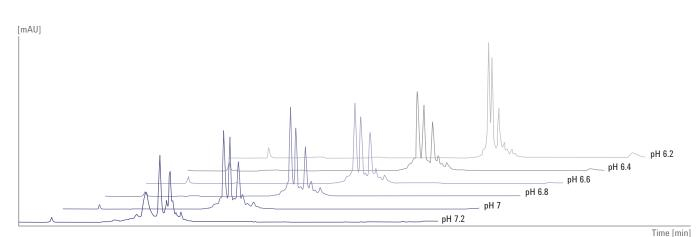
Using dynamically mixed four-component gradients, calculated by Buffer Advisor software, shortened and simplified the workflow for pH scouting significantly.
