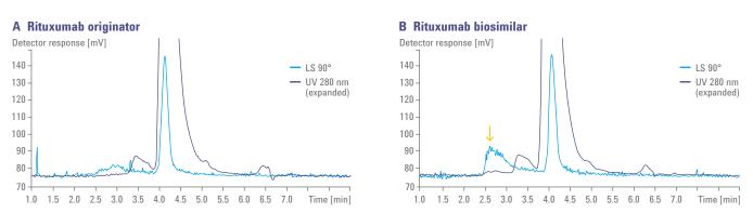
Comparison of LS analysis rituximab innovator (A) and rituximab biosimilar (B) run at 150 mM sodium phosphate, pH 7.0. Light scattering detection proved more responsive to higher-order aggregates.
