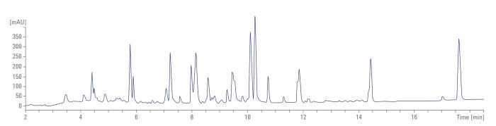
Analysis of P128 digest using an AdvanceBio Peptide Mapping column, 3.0 mm x 150 mm, 2.7 µm at a flow rate of 0.6 mL/min flow rate.
