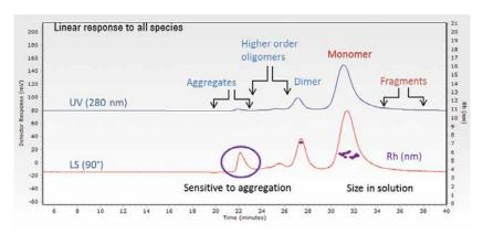
The light scattering detector shows much greater sensitivity to the aggregation present in mAb.
