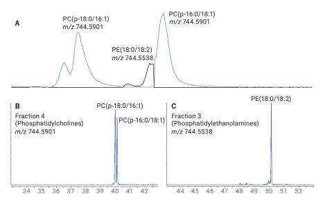
**Figure 6.** Extracted ion chromatogram (positive ionization) for selected PEs and PCs in a plasma sample. (A) shows the one-dimensional RPLC separation, (B) traces show the results for the multiple heart-cutting analyses where PEs and PCs are separated in the first dimension HILIC separation.
