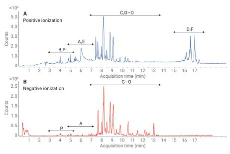
**Figure 2.** Total ion chromatogram (positive and negative ionization) for the analysis of a plasma sample with the second dimension RPLC mode (flow: 0.5 mL/min, gradient: 0 to 5 minutes: 60 to 80% B, 5 to 17 minutes: 80 to 100% B).
