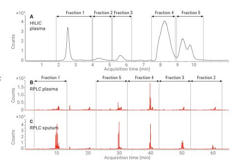
**Figure 5.** Total ion chromatogram (negative ionization) for the analysis of a plasma sample with the first dimension HILIC mode and BPC (–) of the multiple heart-cutting analyses of plasma and induced sputum.
