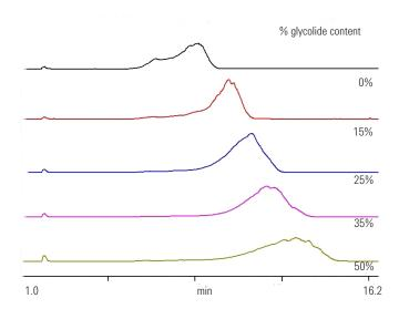
Figure 19. Chromatograms of poly(lactide-co-glycolide) copolymers at different concentrations of tetrahydrofuran
