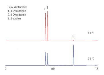
Figure 16. Low temperature operation of the Agilent ELSD shows the true concentration of a pharmaceutical formulation
