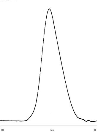
Figure 3. Raw data chromatogram of a broad-distribution polyvinyl pyrrolidone in an aqueous solvent with Agilent PL aquagel-OH columns
