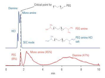
Figure 6. Amine-modified polyethylene glycol before (lower) and after (upper) neutralization with hydrochloric acid
