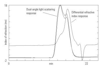
**Figure 12.** Refractive index, and 90° and 15° light scattering data for gelatin, on an Agilent PL aquagel-OH MIXED-H two-column set
