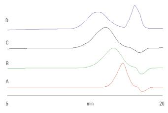
Figure 8. Chromatograms of four pectin samples on Agilent PL aquagel-OH MIXED columns
