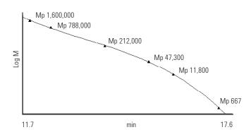
Figure 7. Pullulan standard calibration curve for the Agilent PL aquagel-OH MIXED-H 8 um column
