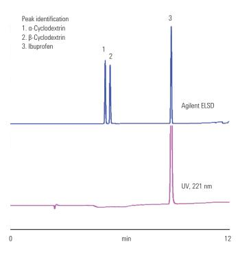
Figure 15. The presence of cyclodextrins revealed by Agilent ELS detection
