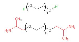
Figure 4. Structure of original (upper) and modified (lower) polyethylene glycol
