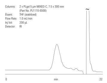
**Figure 17.** The broad molecular weight distribution of a polycaprolactam revealed by gel permeation chromatography with Agilent PLgel MIXED-C columns (system peak has been cut)
