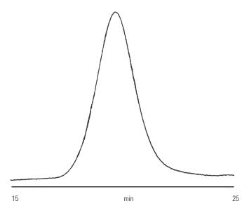
Figure 13. Analysis of cellulose acetate using Agilent PLgel 10 µm MIXED-B columns
