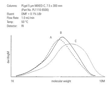
Figure 21. Analysis of three samples of hydroxyethyl cellulose using Agilent PLgel 5  $\mu m$  MIXED-C columns
