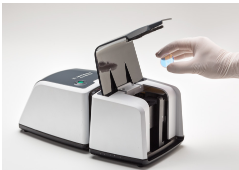
Cary 630 with the 45 degree SRA, which sits within the transmission module.
