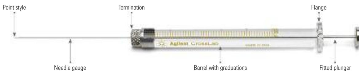
Syringe terminations at the end of the syringe barrel function as the interface between the syringe and its mating connection such as the needle. Terminations are offered in a number of different needle and connection configurations to accommodate a broad range of applications.
