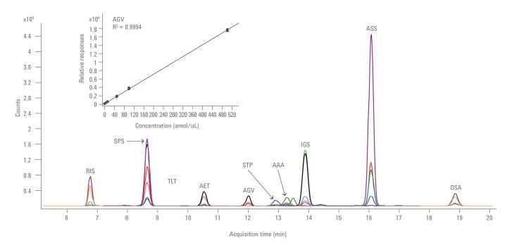
MRM chromatograms for phosphopeptides (1 fmol) from trypsinized *E. coli* lysate (150 ng) using ProtID-Chip equipped with a 160 nL trap. (Inset) Calibration curve of the peptide AGVIQTSTEHS\*FSK illustrates excellent linearity, dynamic range, and reproducibility with an on-chip LOQ of 1 amol.
