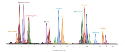
Forensics test mixture results acquired using 25 pg of each compound injected on-column to the new 6420 Triple Quadrupole LC/MS System.
