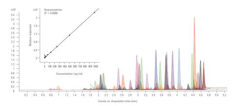
Extracted ion chromatograms of 174 transitions used in the simultaneous quantitation of drug compounds (amphetamines, benzodiazepines and opiates). A wide linear dynamic range was achieved with routine precision of less than 10% RSD in urine samples. (Inset) Calibration curve for buprenorphine demonstrates linearity from 4 to 1000 ng/mL.
