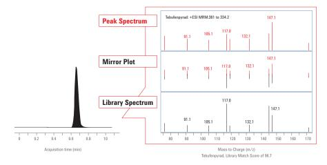
The above below, generated with data gathered using an Agilent 6460 Triple Quadrupole, shows how the acquired mass spectrum (upper window) can be compared to a stored library spectrum (bottom window). The mirror plot in the central window simplifies the comparison between the sample and library spectra. An excellent library match score of 96.75 confirms the identity of the compound.
