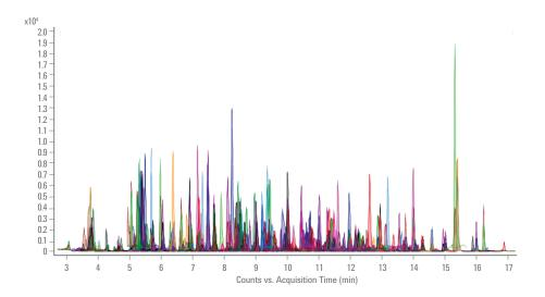
MRM chromatograms of 20-fold dilution of 250 pesticides spiked into black tea at 10  $\mu$ g/kg with insert demonstrating the pesticide LLOQs and IDLs.
