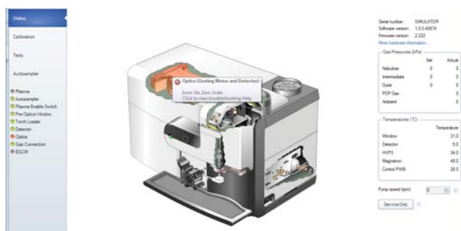
Figure 11. View the interactive Instrument Status page to check the current status of the instrument and identify causes of problems
