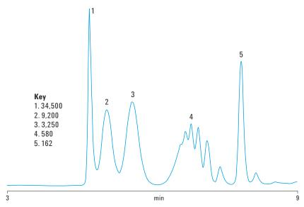
Figure 1. Separation of low molecular weight polystyrene standards on an Agilent PLgel 3  $\mu$ m MIXED-E column.
