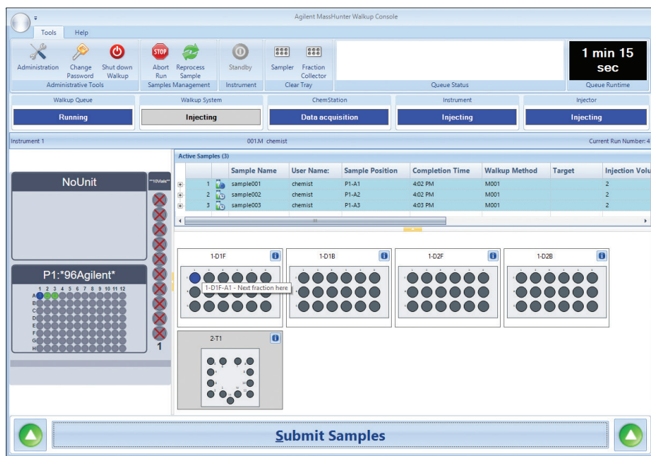
Figure 6. Agilent MassHunter Walkup Status screen showing fractions collected with 1290 Infinity II Preparative Open-Bed Fraction Collector and 1260 Infinity II Preparative Valve-Based Collector.
