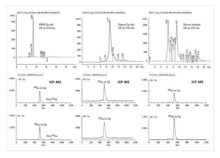
Figure 1. SEC-ICP-MS chromatograms for Cp standards and serum sample. X axis: retention time in minutes for UV detection and in seconds for ICP-MS; Y axis: absorbance at 215 nm for UV chromatograms and total counts for ICP-MS chromatograms.
