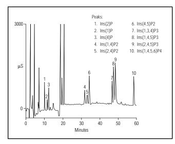
*Figure 6* Separation of inositol mono-, di-, tri- and tetraphosphates in one injection.
