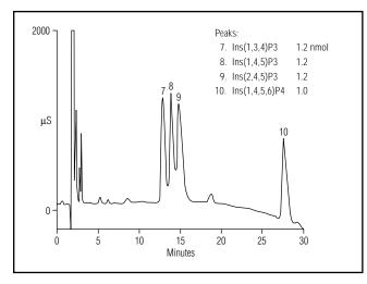
*Figure 5* Separation of inositol triphosphates and an inositol tetraphosphate.
