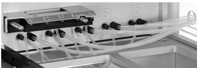
Figure 62. All the solvent tubes in position.
