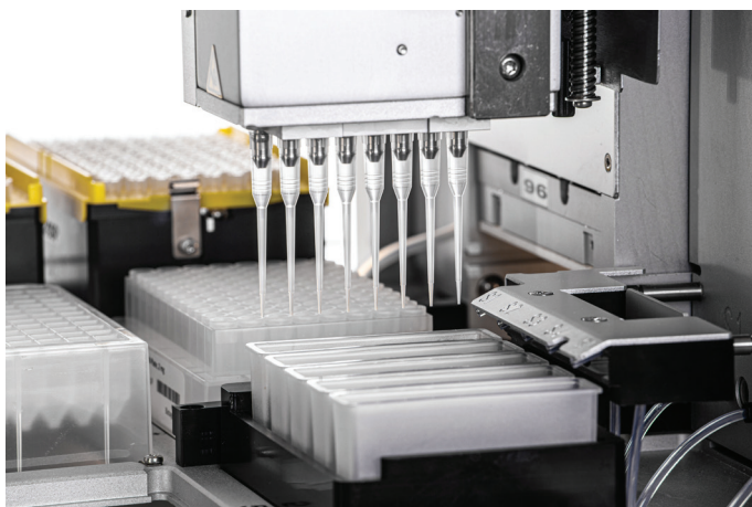
Figure 1. The robot is aspirating solvent from the solvent reservoirs inside the system using disposable pipette tips.
