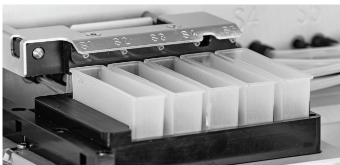
Figure 34. The solvent feeder in position to deliver solvent to the five reservoirs in position 5 on the working area.
