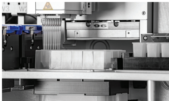
Figure 4. When running a DFE method, wash and elution plates are loaded into the carousel. By removing the plate/rack frame in position 3 on the working area, the carousel plates can be moved up into a position where the pipette and DFE column tips can access them.
