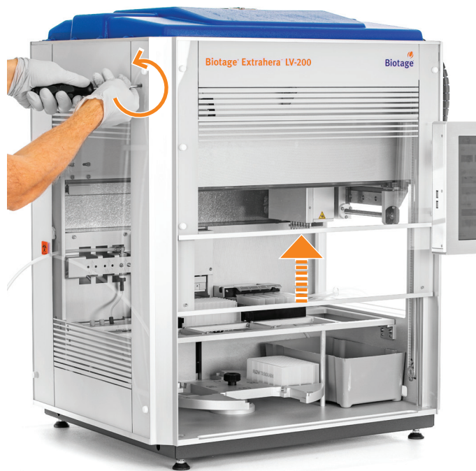
Figure 8. Open the door manually by turning the screw counterclockwise using the T25 Torx screwdriver supplied with the system.
