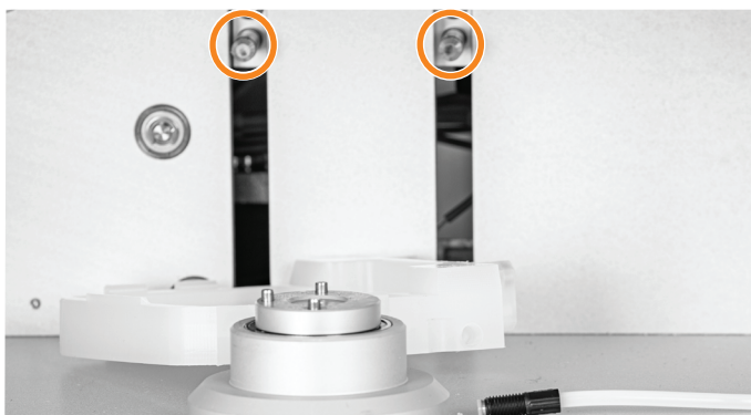
Figure 59. Removing the extraction waste collector. In this image, the carousel has been removed, which is not required. The mounting pins are highlighted.
