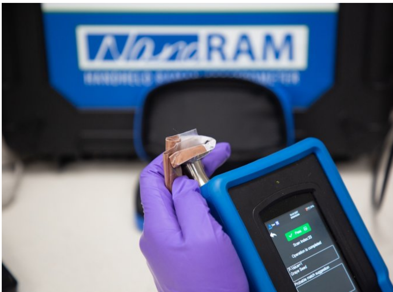
Figure 2. Analyzing grape seed extract with 1064 nm laser with point and shoot adapter.
