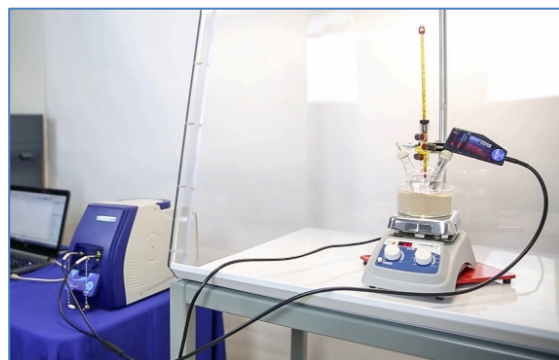
Figure 2: Portable i-Raman ® Plus spectrometer with fiber-coupled immersion probe inserted in reaction
