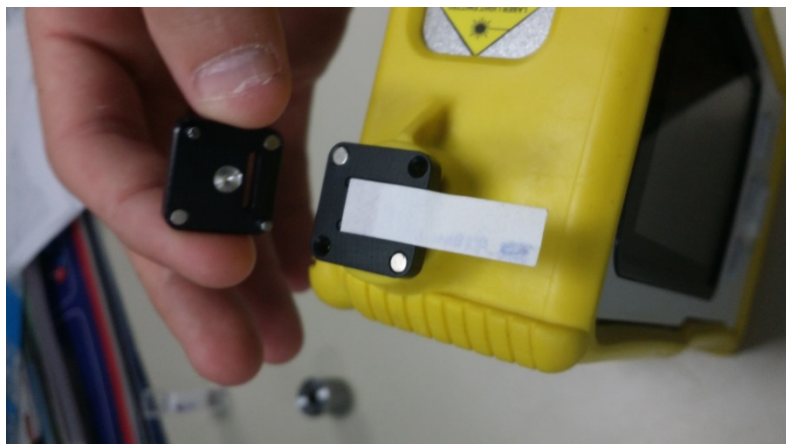
Figure 2: SERS test sample placed in TacPac adaptor for measurement.
