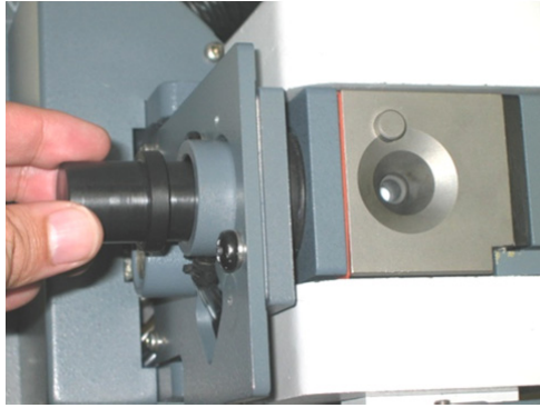
Figure 4. Inserting the probe to check workhead alignment
