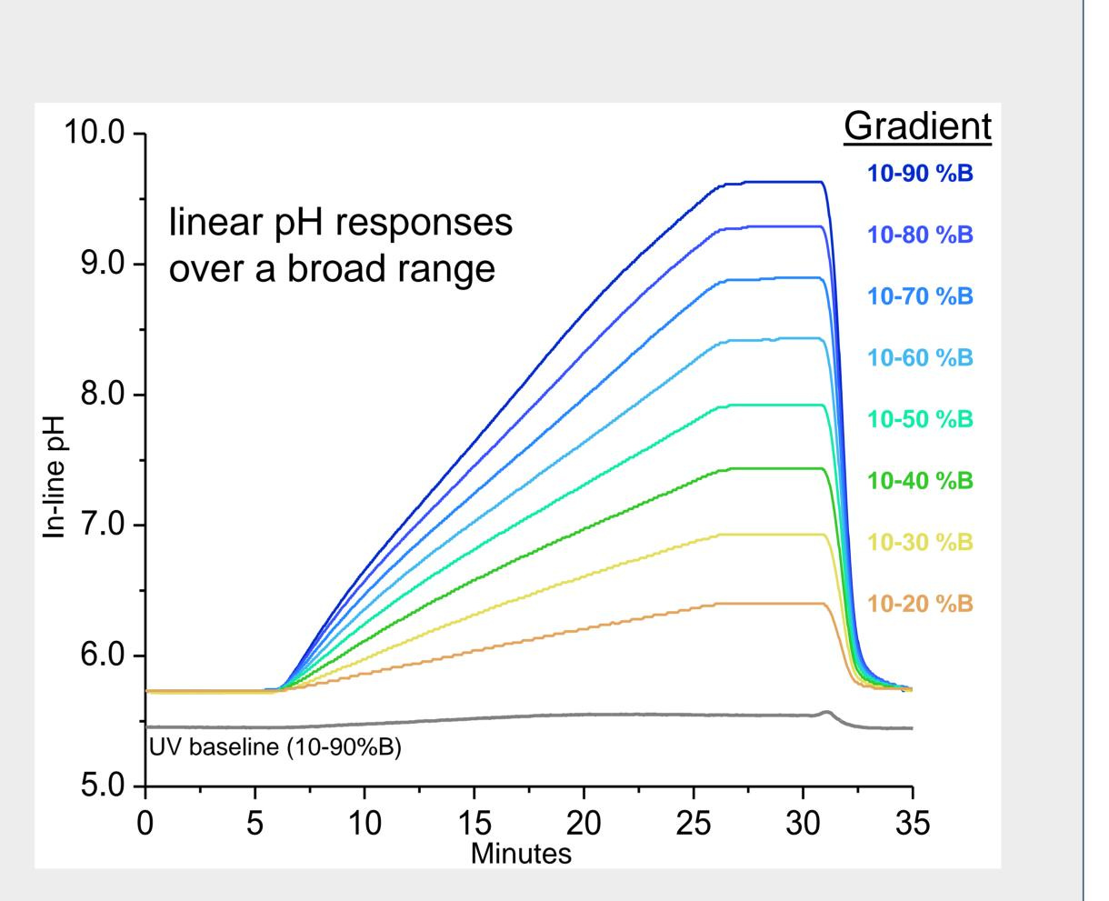
In-line pH measurements of the IEX pH buffers were observed to have a linear and proportional response over a broad range. This broad coverage enables charge variant analysis of a wide variety of proteins and coupled with optical and MS compatibility, empowers faster development and manufacturing of drug products.<sup>2</sup>
