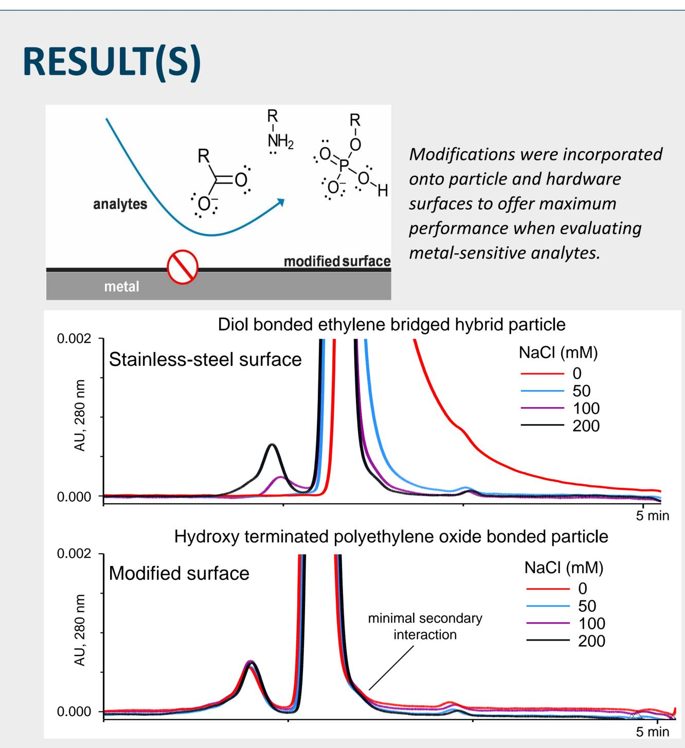
The column with hydroxy terminated polyethylene oxide bonded particles (bottom) shows excellent monomer peak shape across the entire range of NaCl concentrations and no change in aggregate recovery between 50-200 mM NaCl. The stainless-steel column with diol bonded ethylene bridged hybrid particles (top) needed an addition of 200 mM of NaCl to match the same performance.<sup>1</sup>
