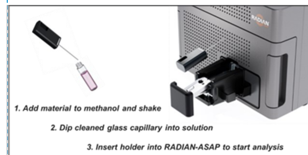
Figure 2. Data acquisition using the RADIAN-ASAP (Waters)
