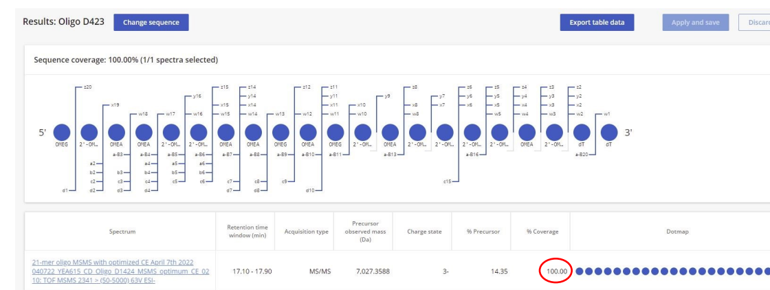
Figure 3. CONFIRM Sequence screenshot showing excellent MS/MS fragmentation coverage (100%) in a dot-map format. The [M-3H] -3 precursor of the 21-mer heavily modified oligonucleotide (m/z = 2342.0) was fragmented using an optimized fixed collision energy (set at 63 V) in the collision cell of a Xevo G2-XS QTOF instrument.
