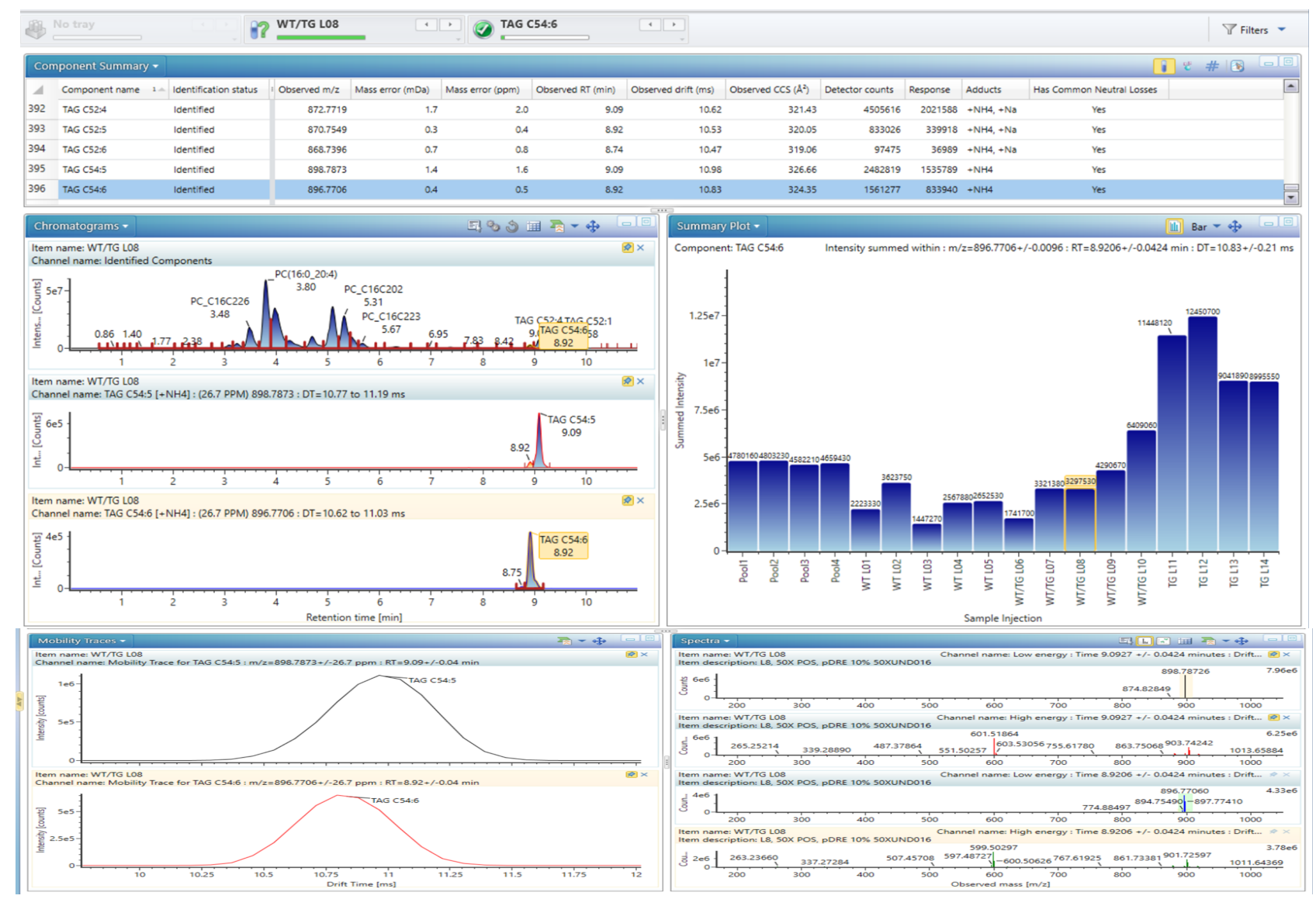
Figure 2. UNIFI™ Summary for Selected TAGs observed in Liver. Tabulated data includes mass accuracy, observed Collisional Cross Section (CCS), and detector counts. Arrival Time Distributions (ATD) and Mobility filtered low and high energy spectra for TAGS C5:4 and C5:6 are shown. Neutral loss is consistent with a C18:2 acyl chain.
