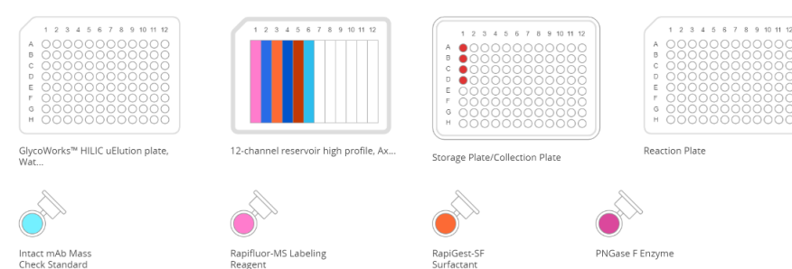
Figure 3: The OneLab workbench setup used for the automated GlycoWorks protocol. Each of the RapiFluor-MS reagents are held in a 1.5 mL tube at the start of the protocol to limit user pipetting. These are then distributed as needed to the reaction plate.
