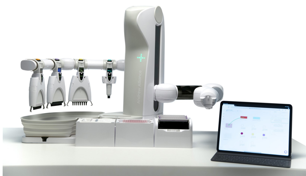
Figure 1: The newly released Andrew+ platform from Andrew Alliance. This system features Sartorius automated pipettors in both single channel and 8 channel formats.
