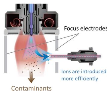
Figure 1 The concept of the IonFocus Unit
