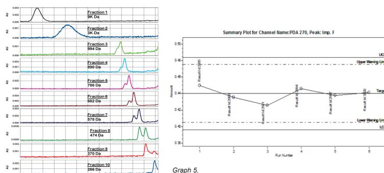
Example of a control chart created using Empower 3 software.
