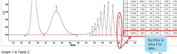
APC integration of polystyrene standards & table of integration values using Empower 3 software.
