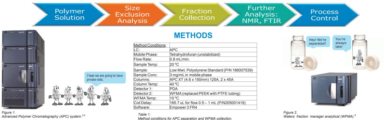
The 10 minute SEC and simplified fraction collection is achieved using a single sample, from a calibration kit, containing multiple low molecular weight polystyrenes. The first procedural step is an SEC analysis for determination of sample peak retention times using the parameters in Table 1. The second step is applying the peak retention times to the fraction collection timing.
