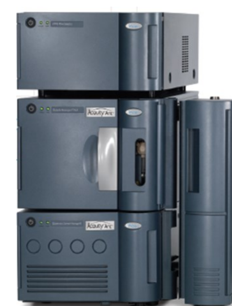
Figure 1. ACQUITY Arc Bio System. The ACQUITY Arc Bio System is a quaternary UHPLC system engineered with bio-inert materials, which are resistant to system corrosion that can be accelerated by the use of high salt mobile phases and pH extremes, while minimizing carryover from undesirable protein system-interactions.
