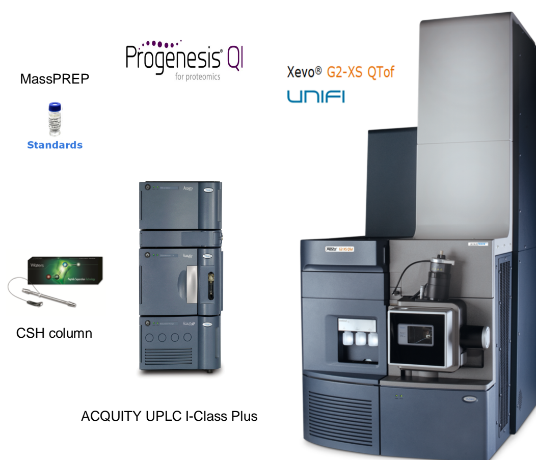
1D LC-MS platform used for HCP identification and quantification in conjunction with Progenesis QI for proteomics software
