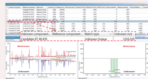
Figure 7: New/differential peaks that are detected when comparing against the reference sample can be reprocessed for identification using the peptide mapping workflow without acquiring new mapping data.
