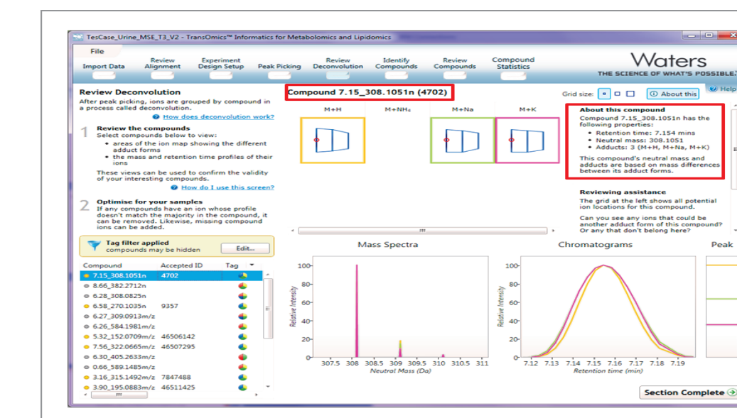
Figure 5. Deconvolution of the adducts from the same compound enables the neutral mass to be determined for more specific database identification and more accurate quantitation.
