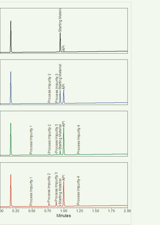
Aliquots of the reaction media are taken from the bench-top reactor and analyzed chromatographically as the reaction progresses. By implementing UPLC as the PAT sensor, information on both the API and low level impurities can be assessed in near real-time.
