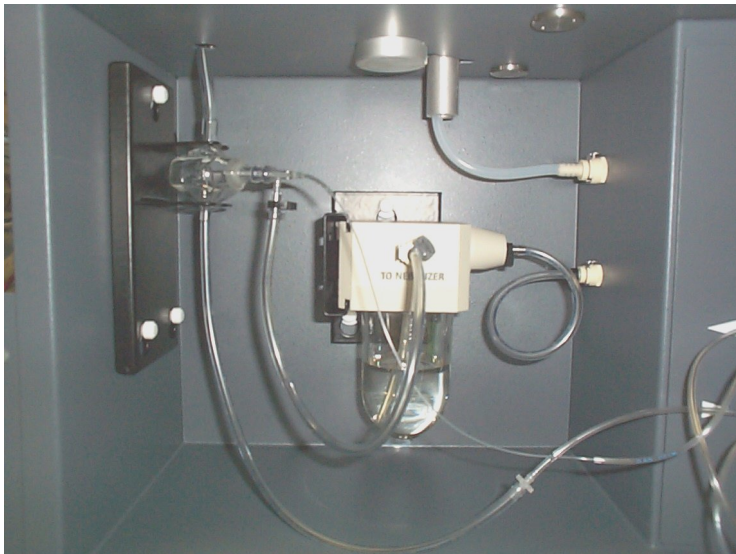
Figure 3. The ASA mounted in the sample compartment of an axial instrument
