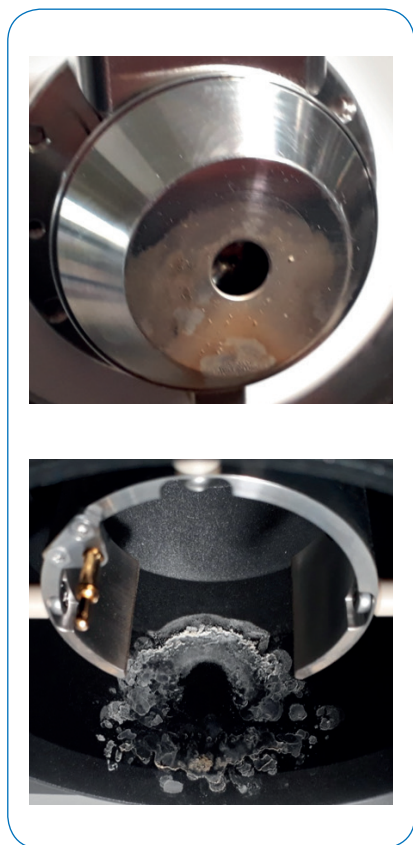
Figure 1: Ion source after > 1100 continuous injections.
