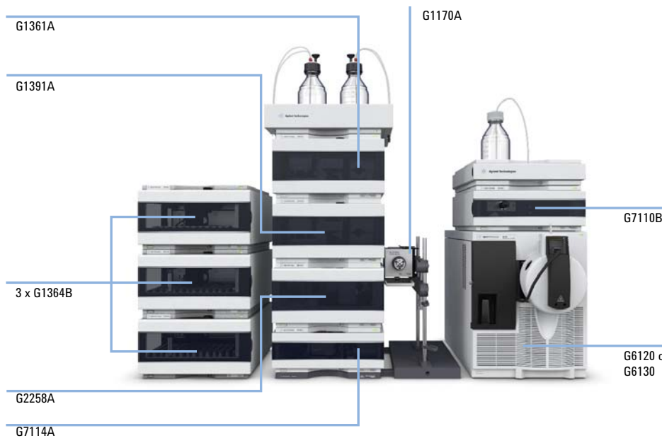
Figure 4 Stack configuration for 1260 Infinity Purification System with UV- and MS-Detection (example shows configuration with 3 FCs in a clustered configuration - optionally available to be stacked in the same order with one FC and only one valve and one valve drive)
