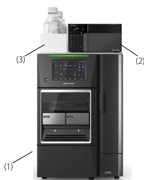
Fig. 1 Appearance of integrated HPLC (1)LC-2070 (2)RID-20A (3)Reservoir tray
